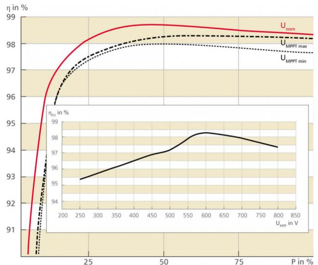
Efficiency values and comparison of the MPPT voltage of the StecaGrid 5503x
